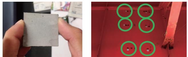
Figure 2. Mortar panels
