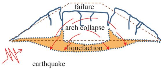
Figure 3. Earthquake induces liquefaction in saturated loose materials within and underneath embankment; consequently, liquefied soil further reduces the confining pressure to the arch abutments; therefore, the abrupt buckling of force chains causes a severe damage to the embankment.
