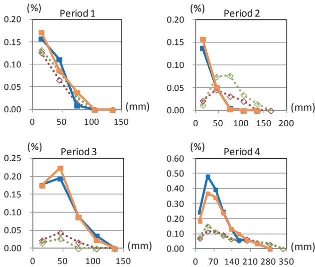
Figure 5. Concentration distribution of Chloride ion in mortar specimens during 4 periods (2015-2017) observation
