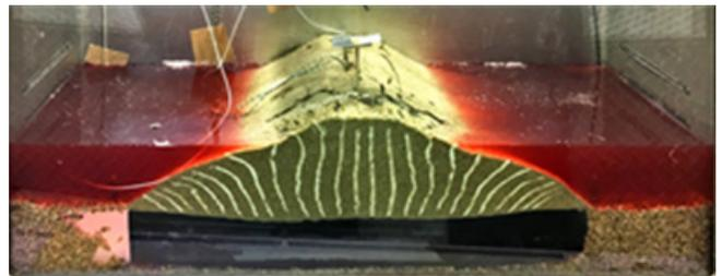
Figure 6. Failure of embankment model after shaking
