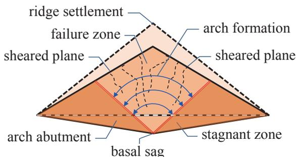
Figure 1. Mechanisms causing sheared plane and failure zone observed in 1G physical model of embankment with basal sag. As arching is ability to transfer load laterally, formation of arch needs relative displacements between the stagnant and mobilized zones.
