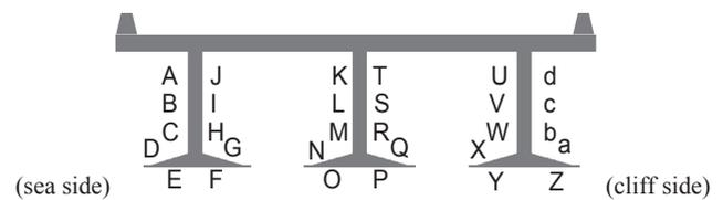
Figure 1. Location of mortar panels
