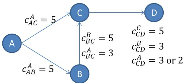
Figure 2. Example network with path-specific link costs
