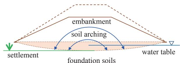
Figure 2. Arches are formed due to basal settlement, causing central pressure drop; hence reducing the resistance against liquefaction.
