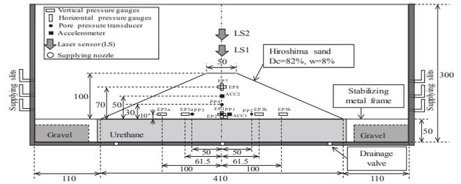
Figure 4. Model configuration and instrumentations
