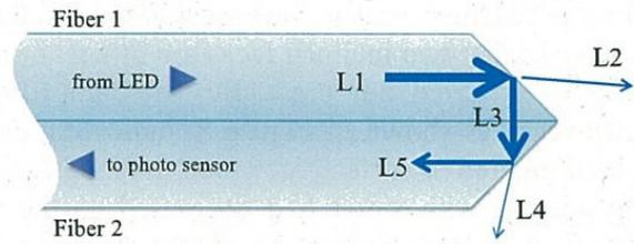
Figure 7. Paths of light around inclined faces of two POFs
