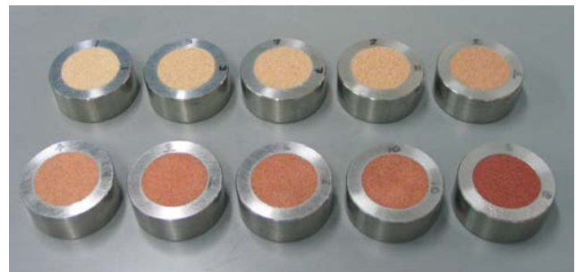
Figure 2. Changes in sand color of sand samples prepared in a laboratory, under varying degrees of NAPL saturation
